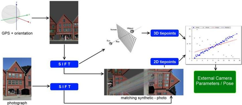
**Fig. 2** Image-to-Geometry algorithm, based on mobile data (left image side), Mutual Correspondence (mid-part) and PnP pose estimation (right side).
