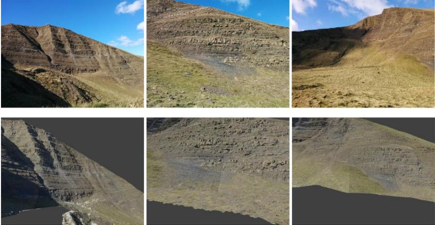
**Fig. 6** Overview of the Mam Tor use case, showing the real-world geologic mobile photographs (top row) and the corresponding Virtual Outcrop rendering from the (error-corrected) GPS-orientation logged initial pose estimate (bottom row).
