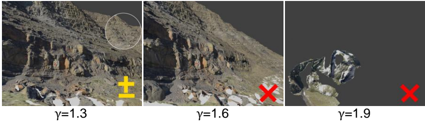
Fig. 7 Registration results for gamma-adapted FAST-SIFT with different \gamma values.
