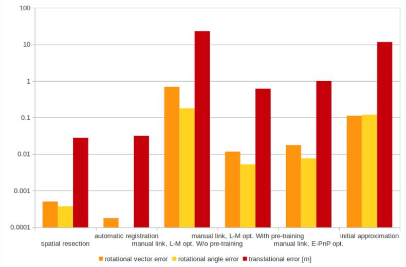
**Fig. 5** Chart giving the average error over 2 Bryggen, compared to the scanner mounting, for vectorial and angular part of rotation quaternion and positioning error (translational).
