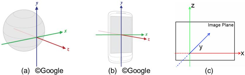
**Fig. 1** Used coordinate systems in the system. The global rotation matrix is given in the mobile coordinate system (a), where the y-axis points to the magnetic north (top-edge of the device in native orientation), the z-axis points away from the center of gravity (out of the device screen), and the x-axis is obtained as yz-axis cross product (b). The used coordinate system aligns with common geographic system, with the xy-plane being ground-parallel while the z-axis delimits altitudes (c).
